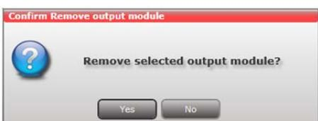
2. Press **Yes** to remove the output module.
